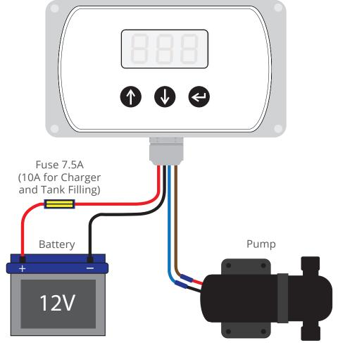
Connect the pump controller in accordance with this diagram. NOTE: only fit the fuse once all connections are made.
