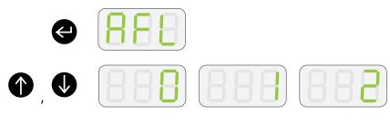
Select the required Autoflush mode with the up or down button. Then press enter to move to the next item.
