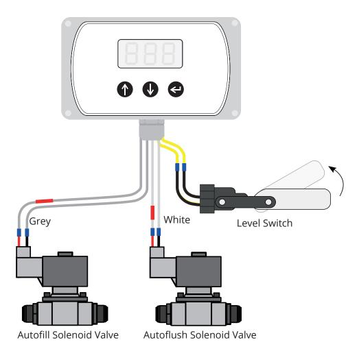
Connect the solenoid valves and level switch in accordance with this diagram. Wire the Autofill solenoid valve using the grey controller wires and the Autoflush solenoid valve using the white controller wires. The level switch should then be connected using the yellow controller wires.
