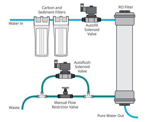
Fit the Autoflush solenoid valve in parallel with the Manual Flow Restrictor Valve, as shown.
