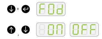
Press up or down to change between on and off. Off will set the controller to 'one time fill'. On will set the controller to 'fill on demand'.
