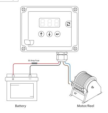
Connect the Reel Winder in accordance with this diagram.
