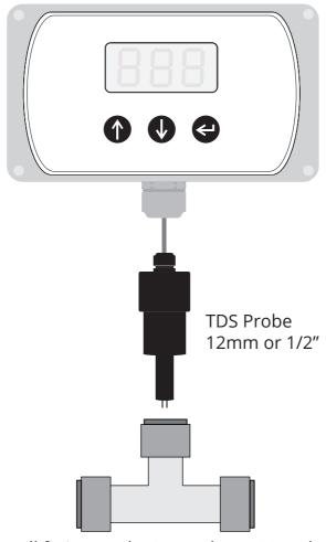
Install fitting on the RO outlet or DI outlet.
