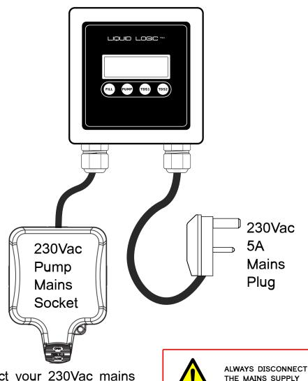
Connect your 230Vac mains powered pump by plugging in to this socket.
