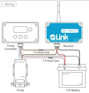
Connect the Stand Alone in accordance with this diagram. NOTE: only fit the fuse once all connections are made.
