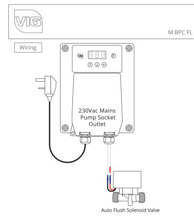
Connect the pump controller in accordance with this diagram.
