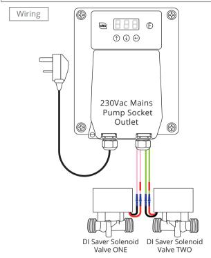
Connect the pump controller in accordance with this diagram.
