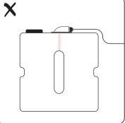
Cut around the drilling template, secure to the top of the tank and drill holes. See Placement Instructions for details on placement. Whilst drilling, prevent swarf from falling into the tank.
