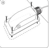
Place the Lumi-Level over the drilled holes, making sure the laser aperture is in the correct orientation, then fasten with screws provided.
