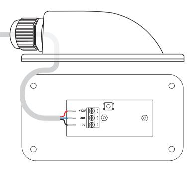
The switch on the Lumi-Level is for the manufacturers calibration only.
