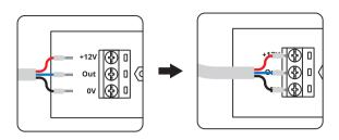
Ensure correct polarity when wiring the Lumi-Level. Failure to do so could result in damage to the unit. If wired incorrectly the unit will not work.
