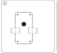
Once the holes are drilled, remove the template and smooth off any rough edges.
