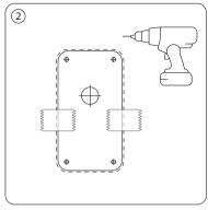
See drilling template for hole sizes. When drilling, prevent the swarf from falling into the tank to avoid any damage to the system.
