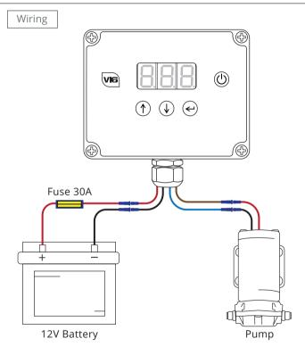
Connect the pump controller in accordance with this diagram. NOTE: only fit the fuse once all connections are made.
