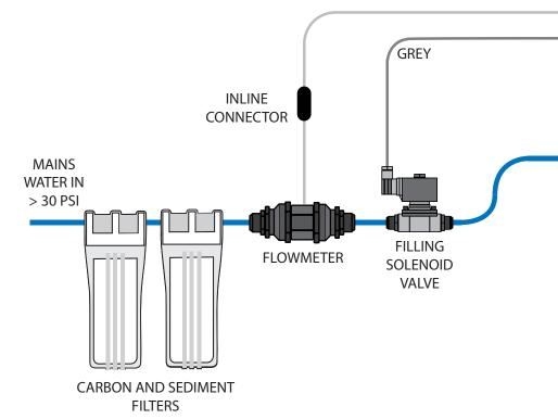
The flowmeter should be fitted between the carbon and sediment filters and the filling solenoid valve as seen above. Connect to the controller using the inline connector.
