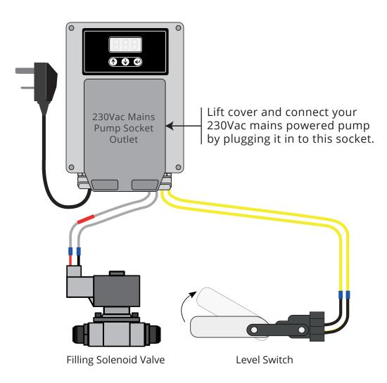
Connect the pump controller in accordance with this diagram and the fitting instructions.
