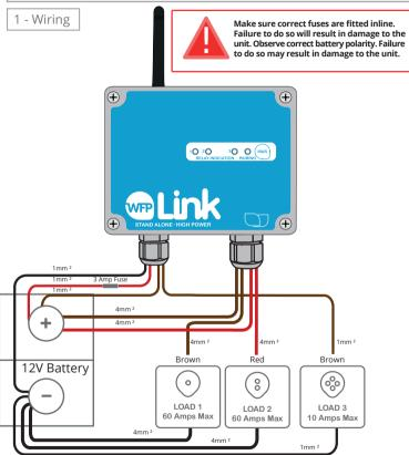
Connect the Stand Alone in accordance with this diagram. NOTE: only fit the fuse once all connections are made.
