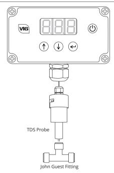
Install fitting on the RO outlet or DI outlet. John Guest 1/2" or 12mm Equal Tee fitting not supplied. Available on request. Specify 1/2" or 12mm probe at time of order.
