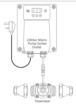
Connect the pump controller in accordance with this diagram.
