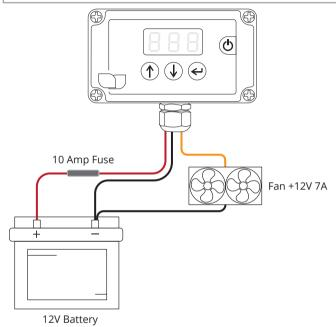
Connect the pump controller in accordance with this diagram. NOTE: only fit the fuse once all connections are made.
