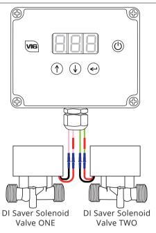
Connect the pump controller in accordance with this diagram. NOTE: only fit the fuse once all connections are made.
