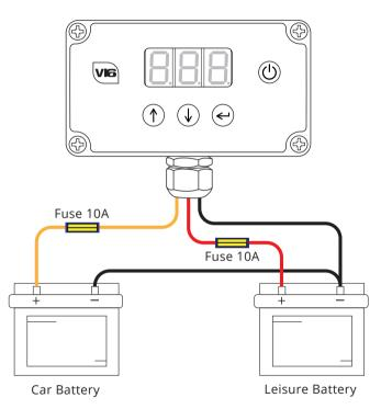
Connect the pump controller in accordance with this diagram. NOTE: only fit the fuse once all connections are made.
