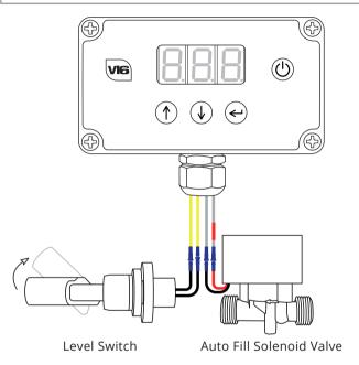
The controller constantly monitors the dead end detection and low battery protection while in fill mode to protect the system. Connect the pump controller in accordance with this diagram.
