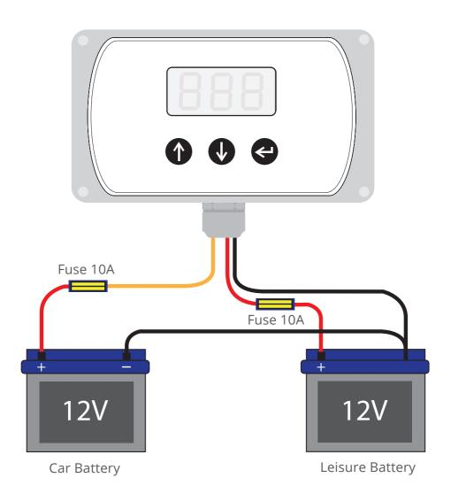
Connect the pump controller in accordance with this diagram. NOTE: only fit the fuse once all connections are made.
