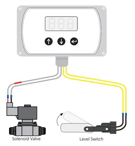
Wire the solenoid valve and level switch in accordance with this diagram.
