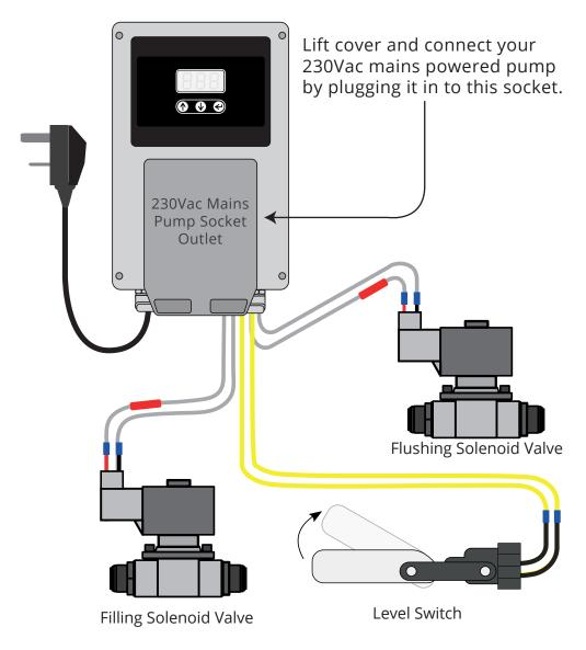
Connect the pump controller in accordance with this diagram and the fitting instructions.
