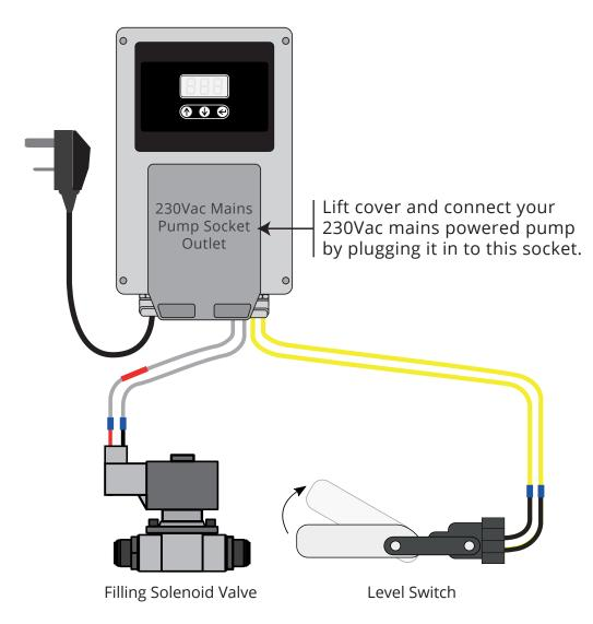
Connect the pump controller in accordance with this diagram and the fitting instructions.
