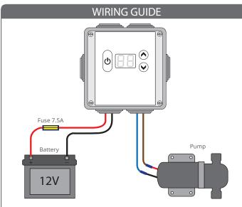
Connect the pump controller as shown above.
